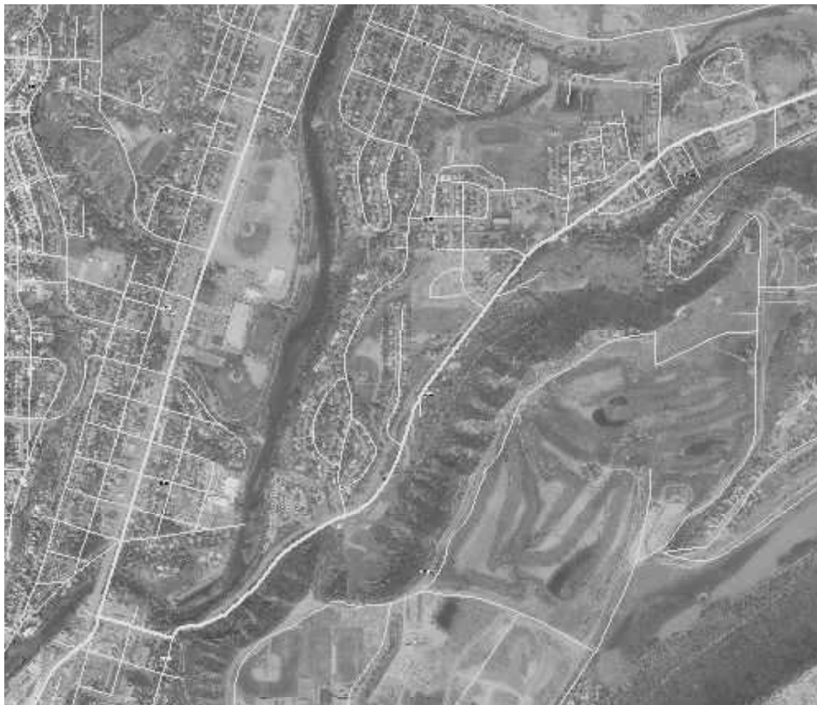
Figure 1. Example showing overlay of roads (bright white lines) on a Digital Orthophoto Quad (aerial photograph). Roads such as the ones shown here were used to spatially allocate county-level mobile source emission estimates.
