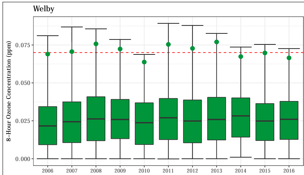
Figure 4.30: 8-hour average O 3 concentrations at the Welby station. The 8-hour standard (0.070 ppm) is shown as a dashed red line. The annual design value (4 th highest daily maximum 8-hour average value) is shown for each year as a green point.
