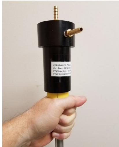
Figure 13.6 – FTS Installation over Stuff
