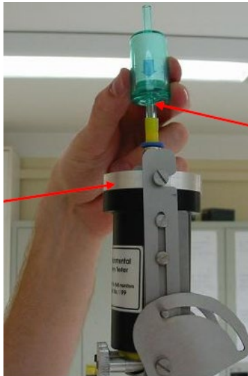
Figure 13.4 – Test Filter Installation
