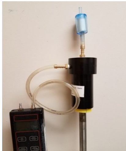
Figure 13.7 – Setup for Zero / Leak Check
